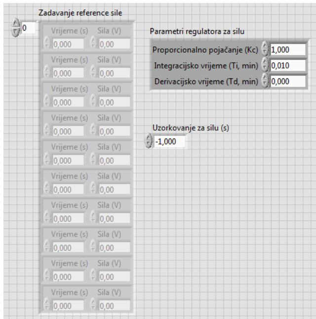
Slika 34. Kontrole PID regulatora i Setpoint Profile ikona na front panelu
