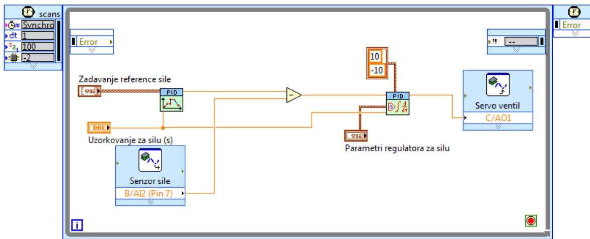
Slika 33. Kreiranje kontrole PID regulatora i Setpoint Profile ikone
