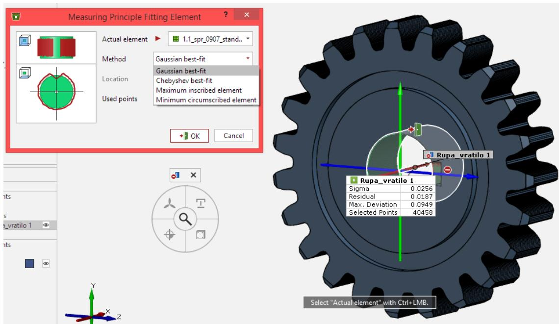
Slika 37 Measuring Principle: Fitting Element - metode
