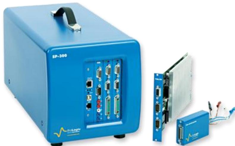
**Slika 9.11.** Potenciostat/Galvanostat BioLogic SP-300 [26]
