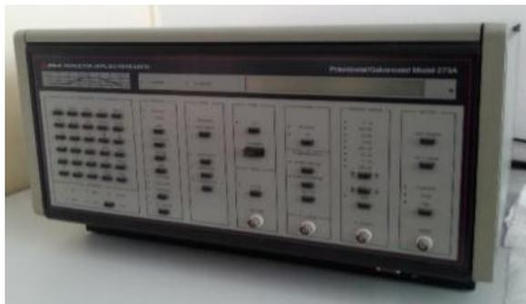
**Slika 9.2.** Potenciostat/Galvanostat Model 273A EG&E
