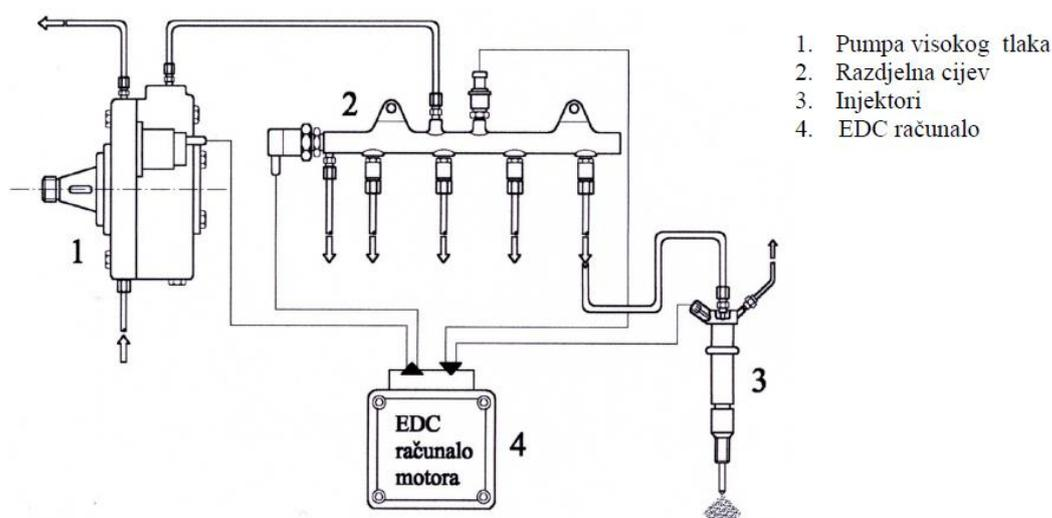
*Slika 35: Dizelski motor s common rail sustavom. [17]*
