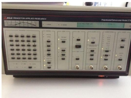
Slika 34. Potentiostat/Galvanostat Model 273A EG&E
