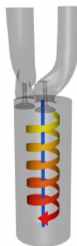
Figure 5 Gas swirl motion inside the IC engine cylinder [13]
