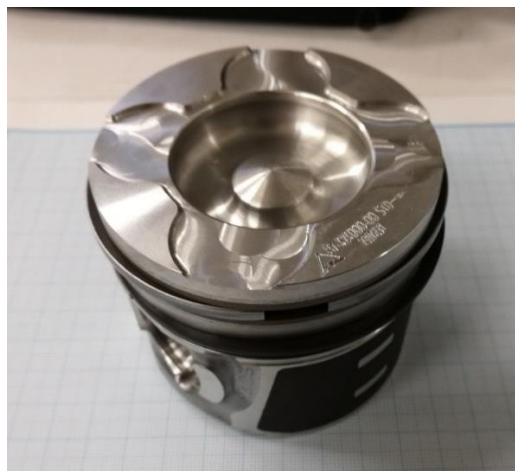
Figure 14 Piston of the observed engine
