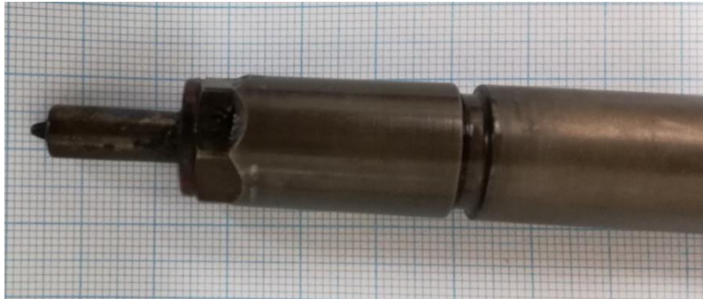
Figure 19 Injector of experimental engine
