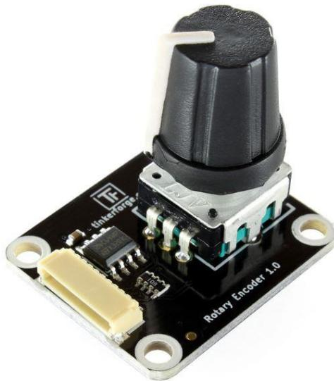
Slika 35. Tinkerforge Rotary Encoder Bricklet
