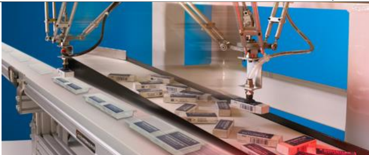
Slika 13 "Pick and place" roboti
