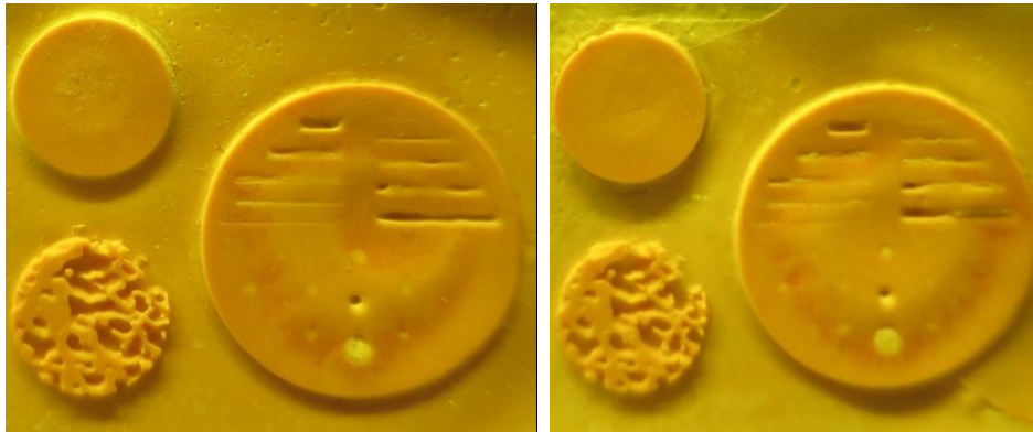
Figure 48. Printing quality of the slurry with 49,7 vol% (left) and 52,3 vol% (right)
