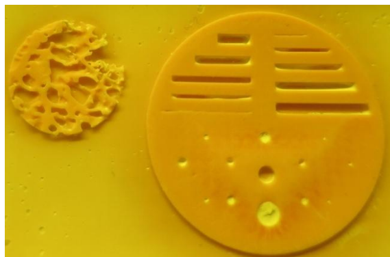
Figure 50. Printing quality of the slurry with D4 (light intensity: 36 mW/cm 2 )
