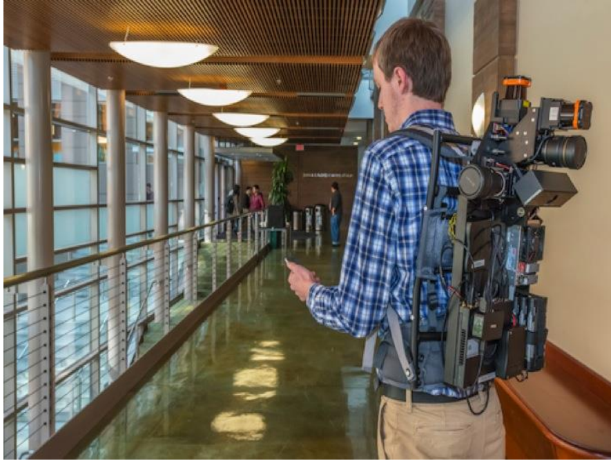
Figure 6 Rapid Building Energy Modeler (RAPMOD) (source:[17])
