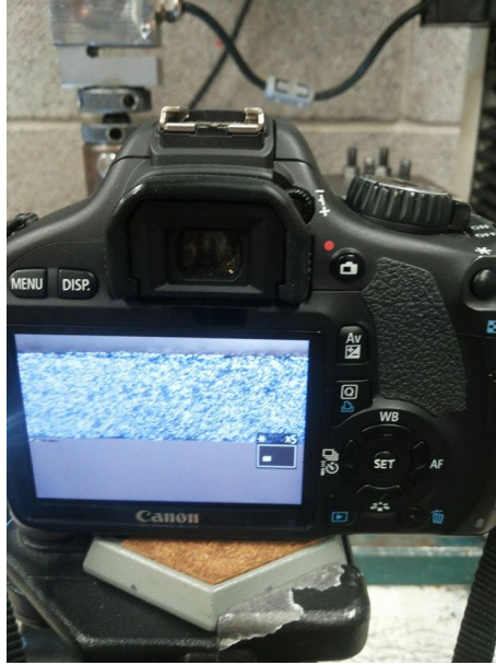
Figure 3.4: Focusing the lens on the speckled sample
