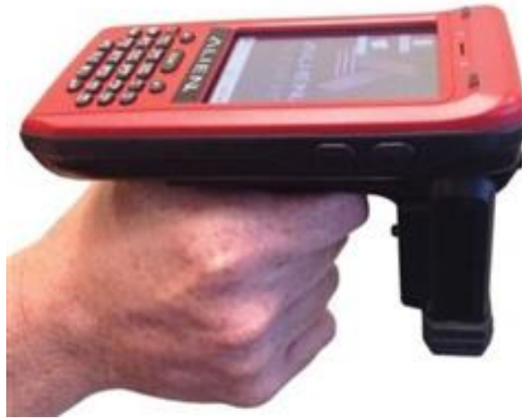
Figure 11-3 Handheld RFID reader with display
