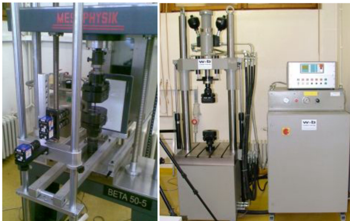
Slika 3 Kidalice: a) MESSPHYSIK BETA 50-5, b) LFV 50-HH; Walter, Bai AG
