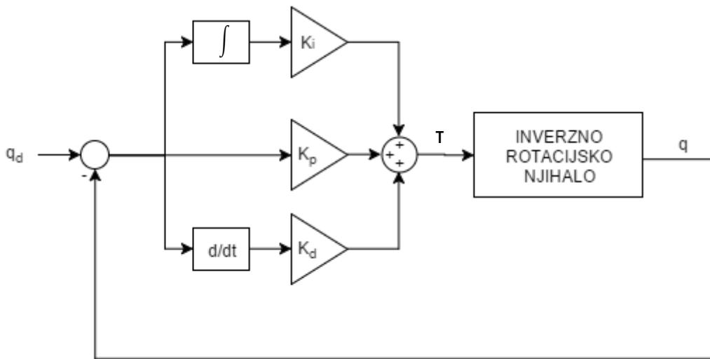
**Slika 3.4 Shema PID regulatora**
