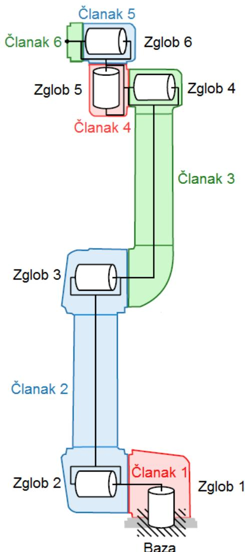
Slika 4.2: Zglobovi i segmenti robota UR5 [13]
