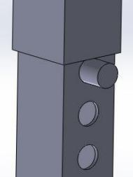
Regulacija visine zaticima<br><input checked="" type="checkbox"/> |
