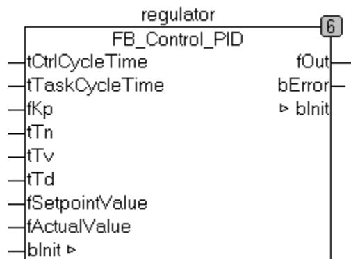
**Slika 6.2 Pid regulator u CFC prikazu**
