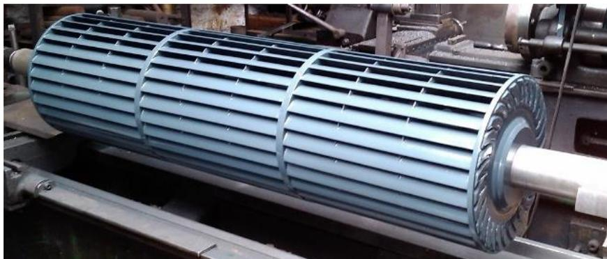
Slika 1 Rotor Ossberger turbine[1]
