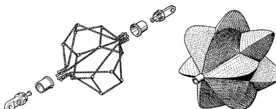
Slika 2.9. ROMAC (ROBotic Muscle ACTuator) pneumatski mišić [6]
