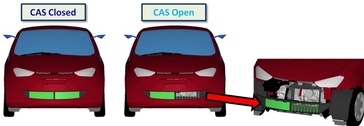
Figure 7.50 CAS closed and CAS open definition
