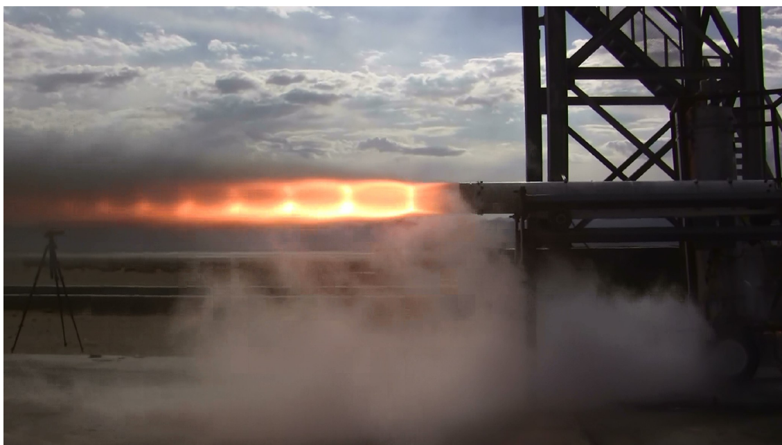
Figure 4.6: Diamond shaped shock waves in the flumes of jet engine [11].
