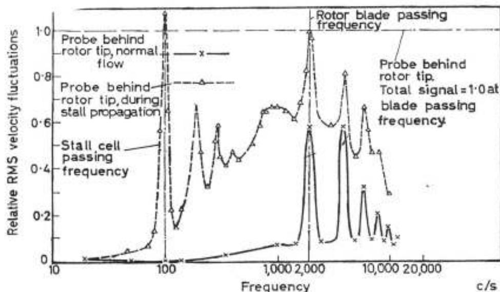
Figure 7.12. Frequencies of velocity fluctuations in compressor during rotating stall (qualitative results only)
