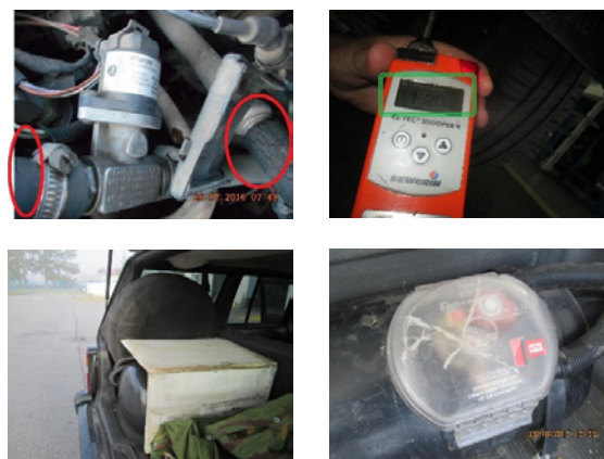
Figure 27: Cracked gas installation pipes and detected gas leakage (top). Inadequately protected gas tank (bottom left) and damaged gas tight housing (bottom right).
