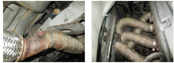
Figure 24: Assembled catalyst and oxygen sensor, and asbestos strips mounted onto the exhaust manifold.
