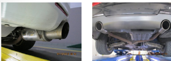
Figure 23: Unapproved type of self-built exhaust silencer and muffler mounted onto the vehicle (left) and unapproved modification – removing the exhaust silencer and muffler from the exhaust (right).
