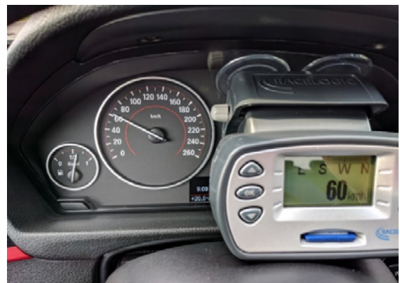
Figure 4: Comparison of vehicle speed measured by the performance meter after the mounting of wheel rims and tires of unapproved dimensions.
