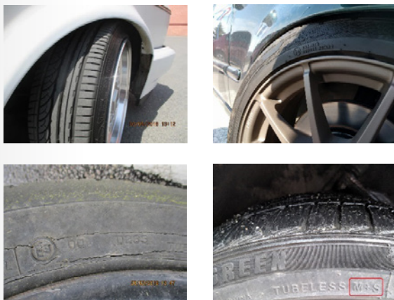
Figure 7: Tires that are too narrow with respect to the width of the wheel rim (top left), tires that get caught under the mudguards (top right), cracked and worn-out tires (bottom left), excessively worn-out tires (bottom right).
