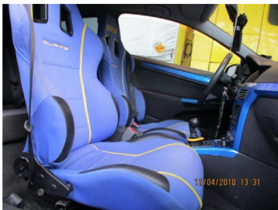
Figure 26: Unauthorized installation of sports seats unapproved for road use.
