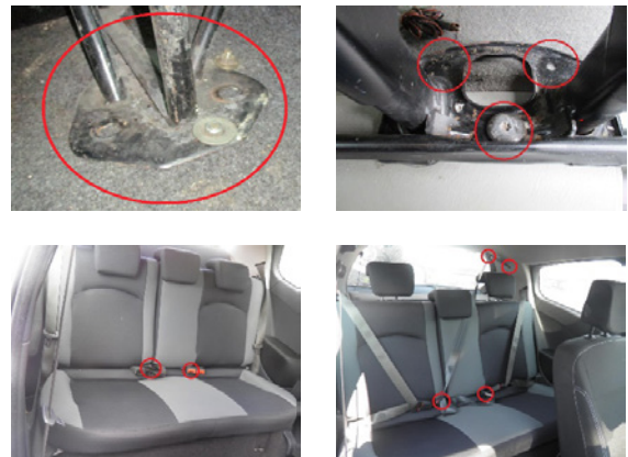
Figure 25: Improperly secured bench seat (top), improperly fitted third seatbelt on the rear bench seat of Renault Clio III (bottom left) and properly fitted third seatbelt on the rear bench seat of Renault Clio III (bottom right).
