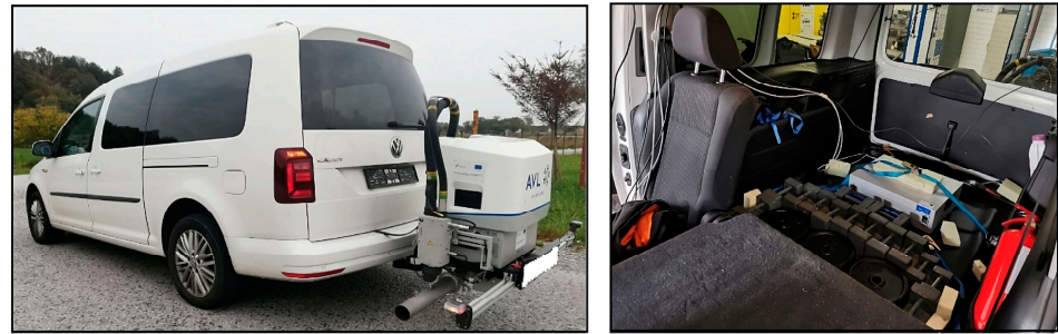
Figure 1. Test vehicle with installed measuring equipment.
