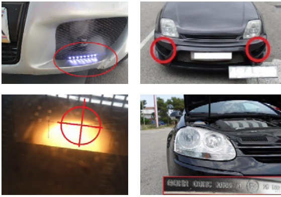
Figure 17: Installation of non-homologated LED daytime running lights (top left), front direction indicators that are not visible – excessive recessing into the bumper (top right), improper alignment of halogen high beam headlights (bottom left), improper installation of xenon lights without ballast, headlamp washers and angle sensors in the headlights intended for halogen light bulbs (bottom right).
