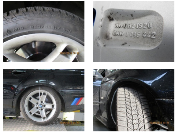
Figure 3: Procedure for testing the mounted wheel rims and tires of unapproved dimensions.
