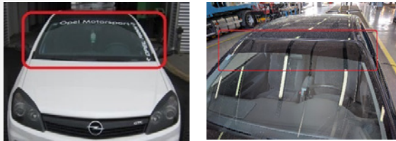
Figure 21: Prohibited application of films and stickers to the windscreen.
