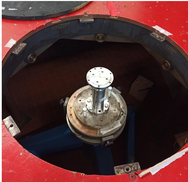
Figure 29. High frequency force balance in the wind tunnel
