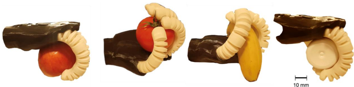
Figure 9: Grasping and manipulation of objects using proposed hand.
