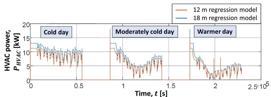
**Figure A2.** HVAC regression model responses for 12 m and 18 m e-bus in heating mode.
