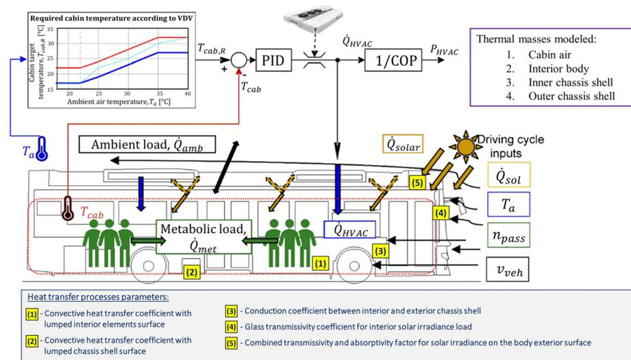
Figure 6. Illustration of HVAC system energy consumption model.
