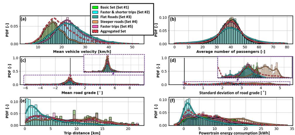
**Figure 13.** Distributions of main features of standard, modified, and aggregate driving cycle sets and the corresponding distribution of powertrain energy consumption (PDF stands for probability density function).
