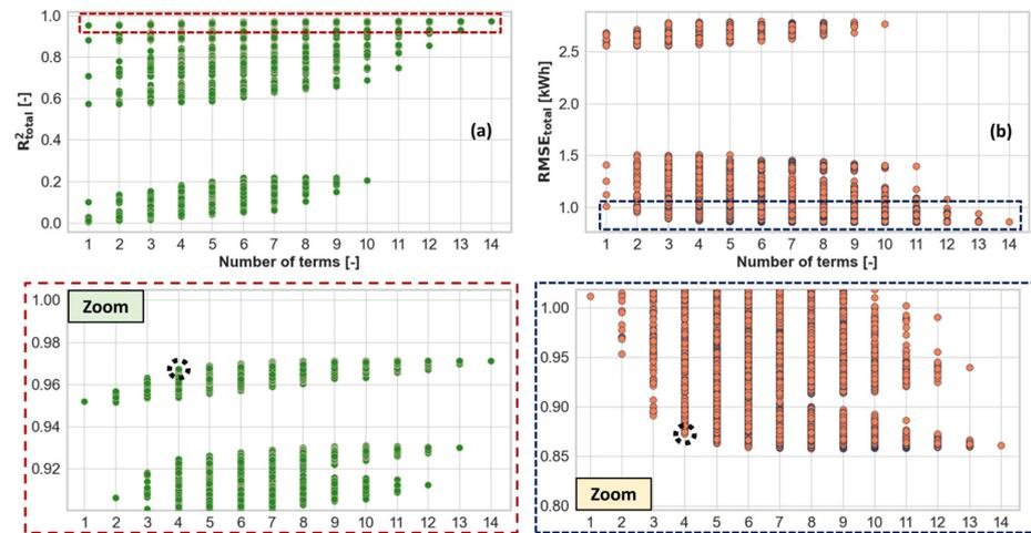
Figure 18. Validation results for the best subset method in terms of R<sup>2</sup> metrics vs. number of predictor variables (a), and RMSE metrics vs. number of predictor variables (b).
