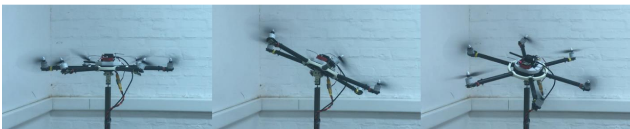
Figure 12. Experimental testing of attitude control on PTX6 for the case of reference state tracking.
