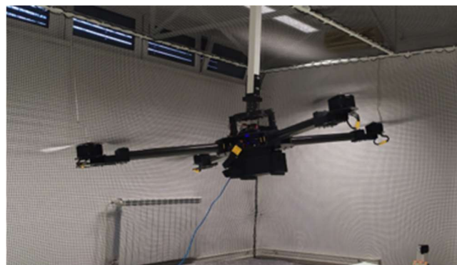
Figure 24. Quadrotor prototype during experimental testing of attitude control.
