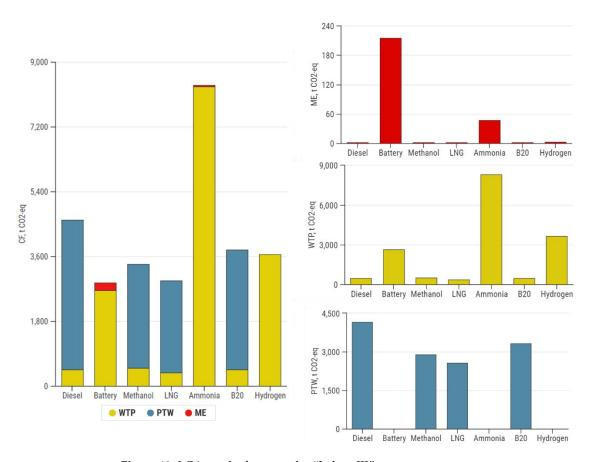
**Figure 13.** LCA results for a trawler "Jadran III".
