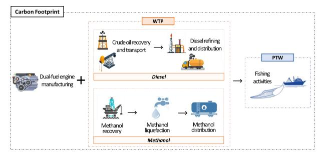
**Figure 7.** The LCA of a methanol-powered trawler.
