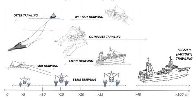
Figure 1. Classification of trawlers by the type of gear and standard length.
