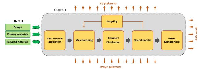
Figure 3. Flowchart of the generalized LCA method.
