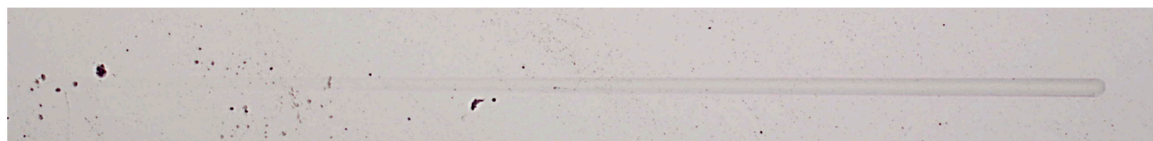
Figure 23. Scratch after testing of the SH-15-TiBN sample.
