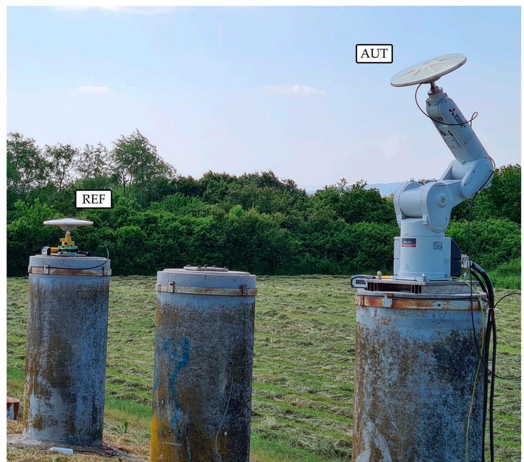
Figure 3. Antenna calibration system set-up at LMMT. Industrial robot Mitsubishi MELFA RV-4FLM-Q with an installed antenna-under-test (AUT) and, in the background, the reference (REF) antenna. Both antennas are of the Trimble Zephyr 2 Geodetic (TRM57971.00 NONE) type without a radome. The baseline length is 5 m. Each antenna is connected to a reference-station-grade Trimble NetR5 GNSS receiver.
