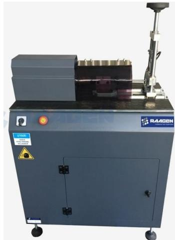
**Slika 5. Raagen Rotating Bending Fatigue Testing Machines [3]**
