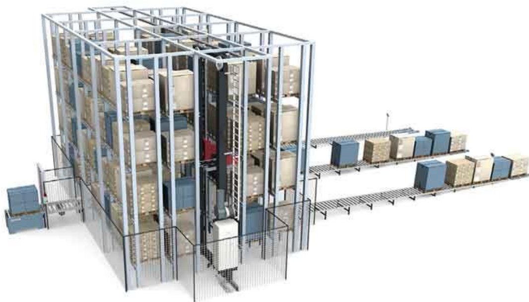
Slika 2. Unit load AS/RS [15]
