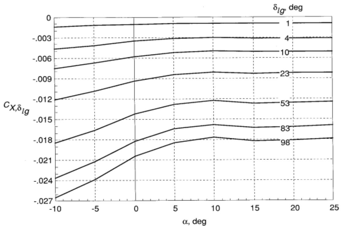
Slika 5. Ovisnost koeficijenta  $C_{X\delta_{lg}}$  o napadnom kutu  $\alpha$  [3]
