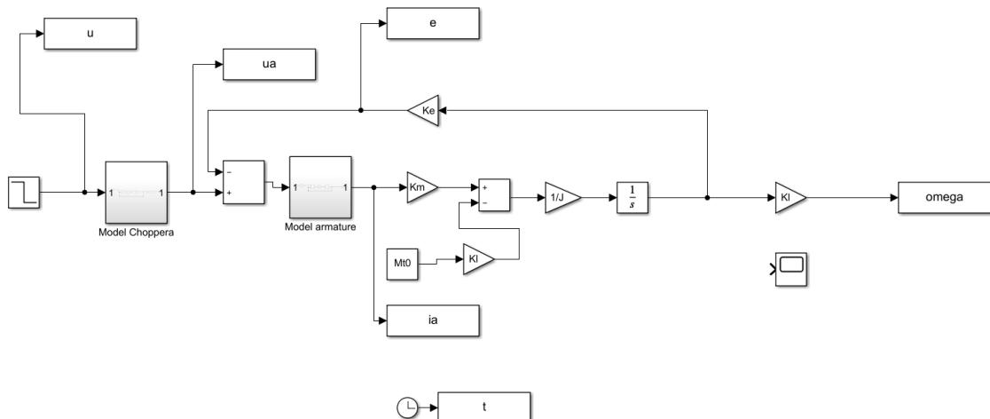
Slika 11 SIMULINK model DC motora
