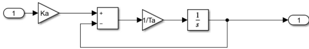
Slika 12 SIMULINK model armature DC motora
