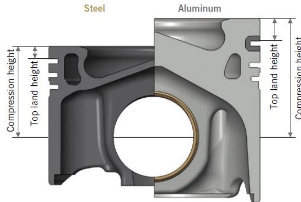
Figure 17. Geometrical comparison of steel and aluminum pistons [8].
