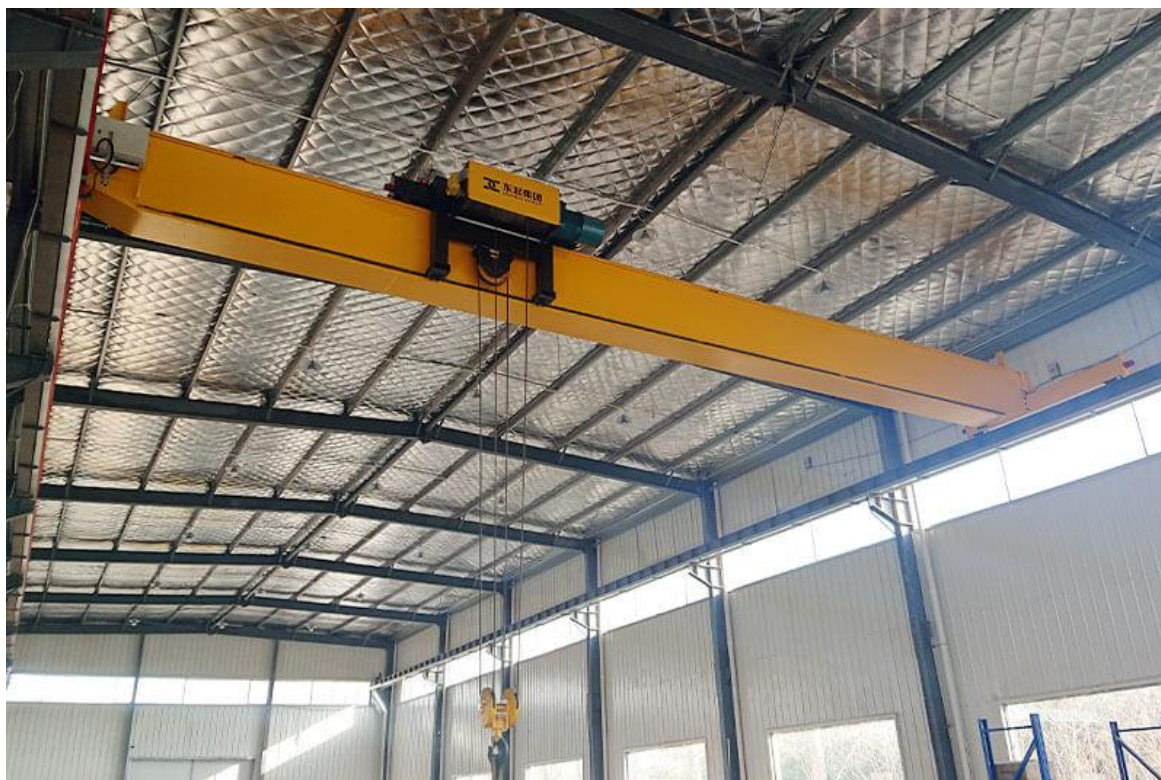
Slika 7. Dongqi group – LDP Low Headroom Singel Girder Overhead Crane
