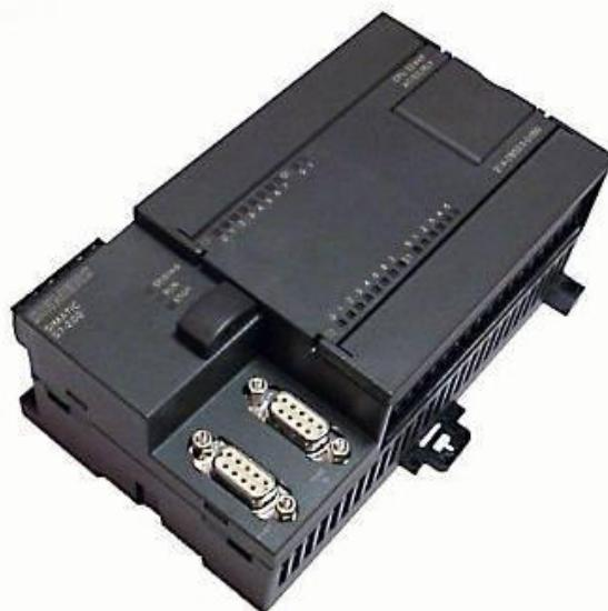
Slika 4.4. PLC - Siemens Simatic S7-200 [15]
