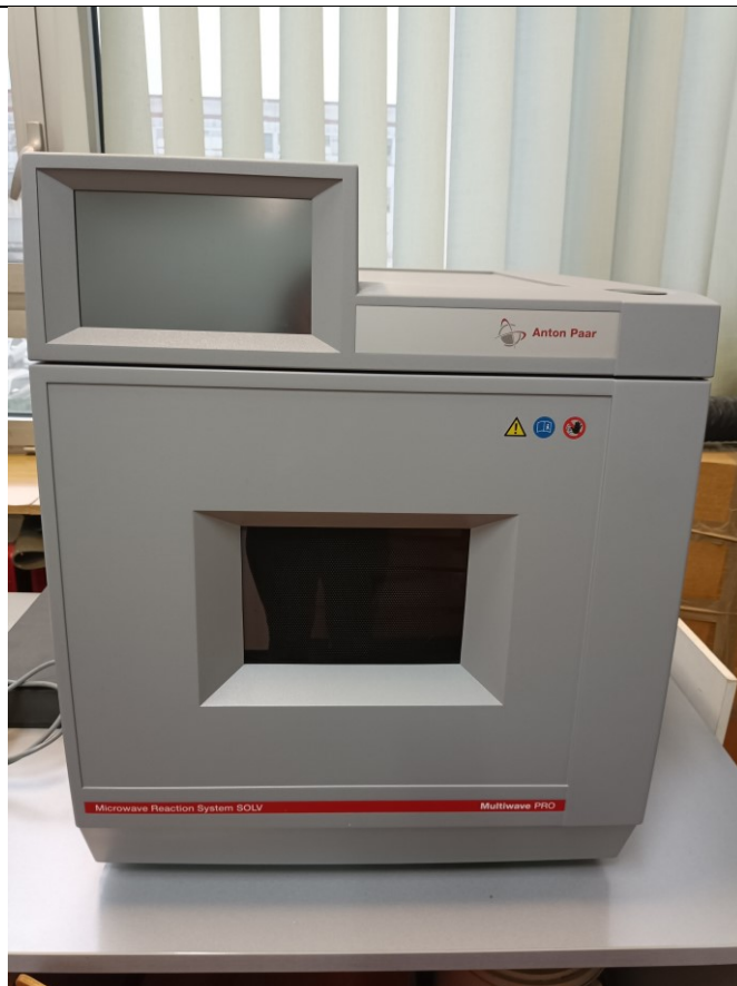
Slika 19. Mikrovalni reaktor (Microwave Reaction System SOLV, Multiwave PRO, Anton Paar, Graz, Austrija)
